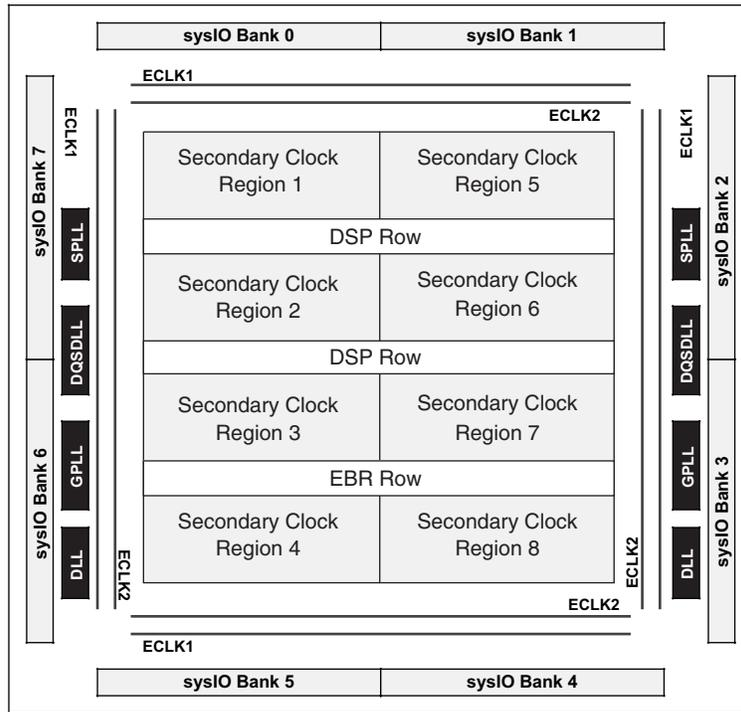
Figure 10-4. LatticeECP2M-50 Secondary Clocks and Edge Clocks
