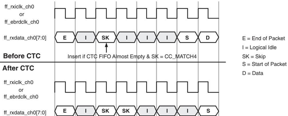
A diagram illustrating 2 byte deletion is shown in Figure 8-11:
