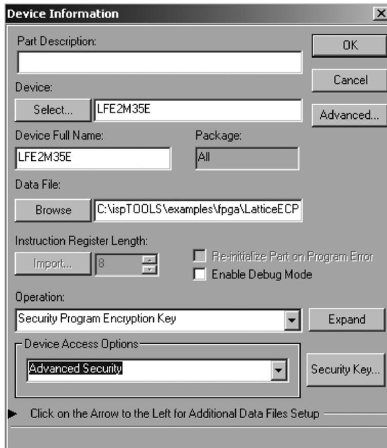
3. Double-click on the line in the chain containing the LatticeECP2. This will open the Device Information window (see Figure 5). From the Device Access Options drop-down box select **Security Mode**, then click on the **Security Key** button to the right. The window will look similar to Figure 16-7.
