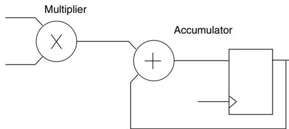
This block diagram can be mapped directly into the sysDSP primitives. Note that if a test point were added between the multiplier and the accumulator, or two output registers, etc. the code could not be mapped into a MULT18X18MACB of a sysDSP Block. Therefore, options that could be included in a design are input registers, pipeline registers, etc.
