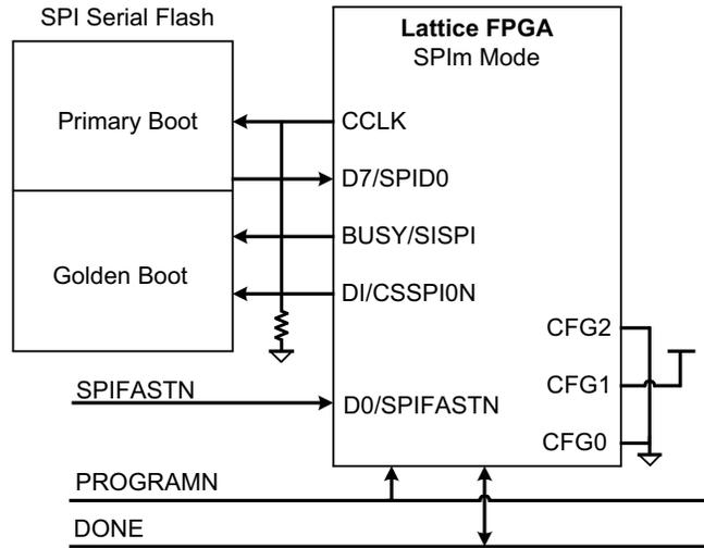
Note: The CSSPI1N pin should not be connected.
