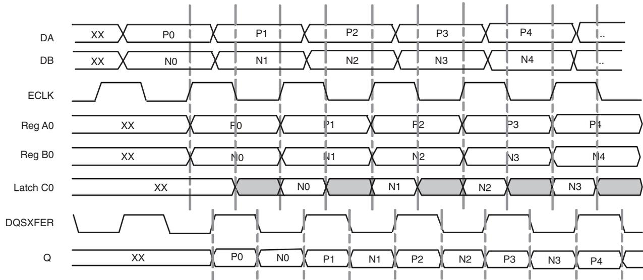
Note that the DQSXFER is inverted inside the ODDRXMA. This will cause the data coming out of the ODDRXMA to be  $-90^\circ$  in phase with the output of the ODDRXC module.
