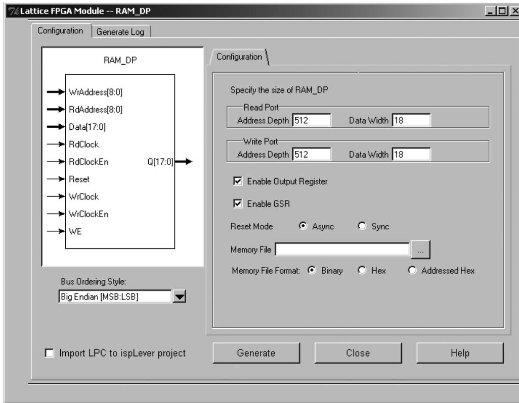
The left side of this window shows the block diagram of the module. The right side includes the **Configuration** tab where users can choose options to customize the RAM\_DP (e.g. specify the address port sizes and data widths).
