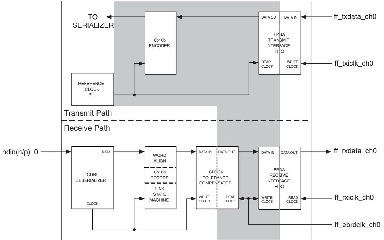
To guarantee a synchronous interface, both the input transmit clocks and input receive clock should be driven from one of the output reference clocks for a PCS quad set to Generic 8b10b mode. Figure 8-16 illustrates the possible connections that would result in a synchronous interface.
