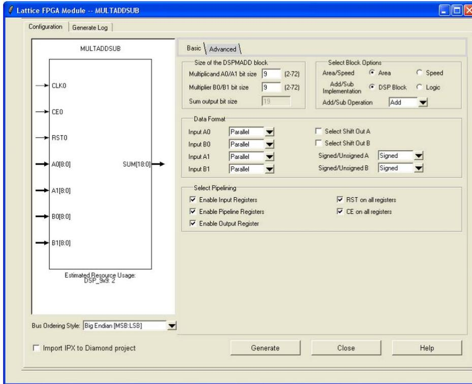
Figure 14-7. MULTADDSUB Mode Advanced Set-up
