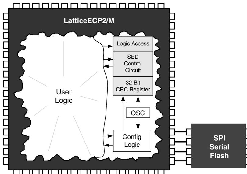
1. Any kind of configuration memory can be used, including the SPI configuration shown.
