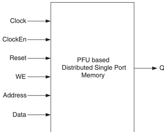
The generated module makes use 4-input LUT available in the PFU. Additional logic like Clock, Reset is generated by utilizing the resources available in the PFU.
