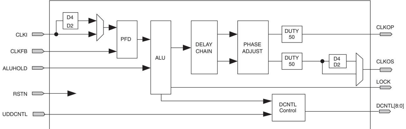
Both clock injection delay removal and output phase adjustment use only the clock outputs of the DLL. Time reference delay and delay match modes use the delay control vector output. Specific examples of these features are discussed later in this document.
