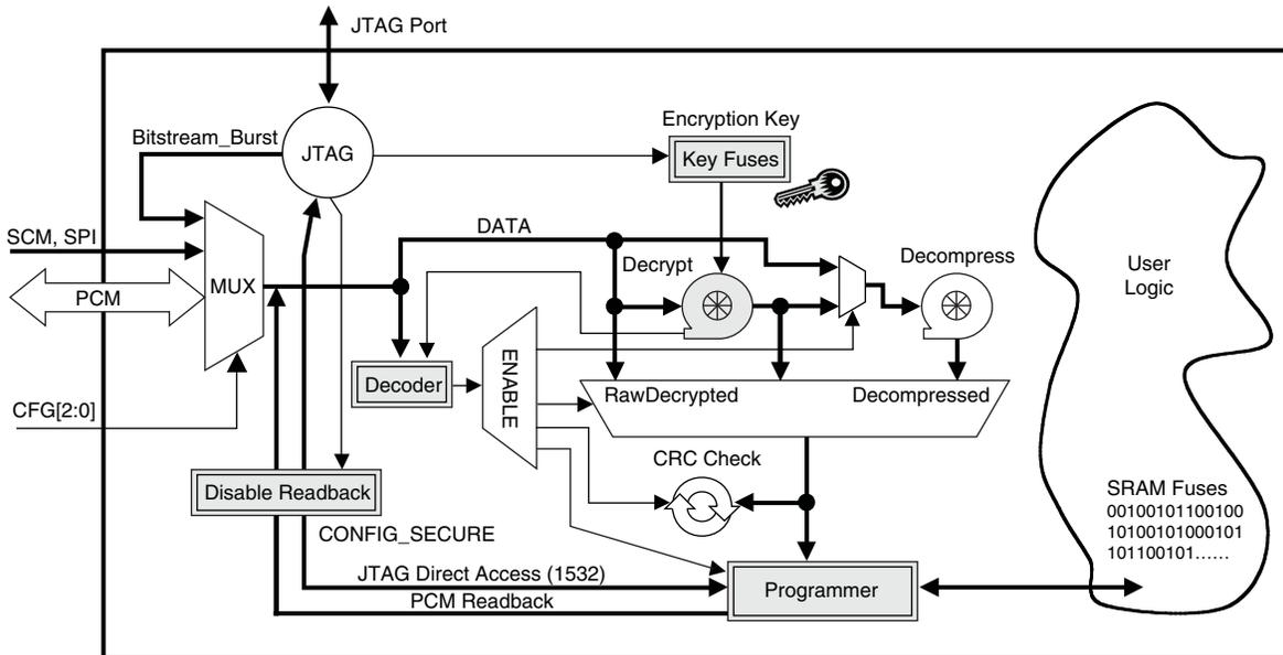
Lattice FPGAs are configured by using the sysCONFIG™ interface or the JTAG interface (see Table 16-1).
