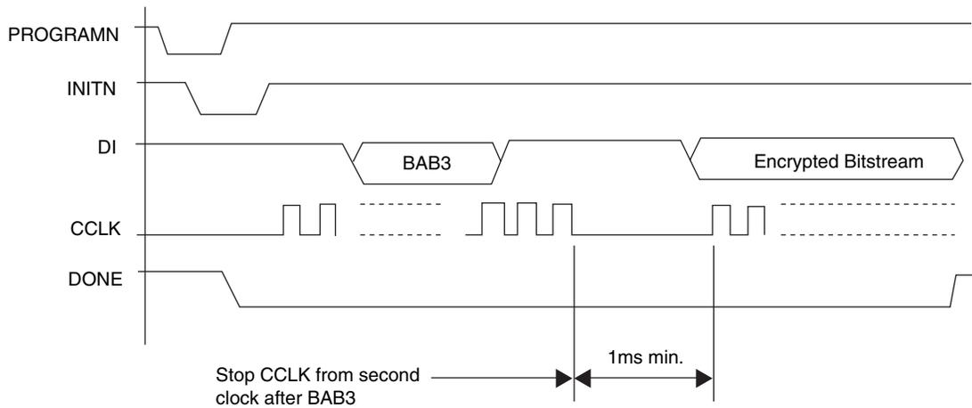
To ensure proper programming when using encrypted bitstreams in SPI mode only a subset of CCLK frequencies are supported. The supported frequencies are shown in the [LatticeECP2/M Family Data Sheet](#).
