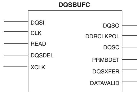
The DQSBUFC is composed of the DQS Delay, the DQS Transition Detect and the DQSXFER block as shown in Figure 12-8. This block inputs the DQS and delays it by 90 degrees. It also generates the DDR Clock Polarity and the DQSXFER signal. The preamble detect (PRMBDET) signal is generated from the DQSI input using a voltage divider circuit.
