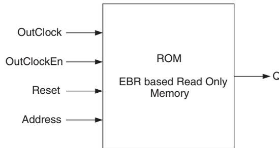
The generated module makes use of these EBR blocks or primitives. For memory sizes smaller than an EBR block, the module will be created in one EBR block. If the specified memory is larger than one EBR block, multiple EBR blocks can be cascaded, in depth or width (as required to create these sizes).
