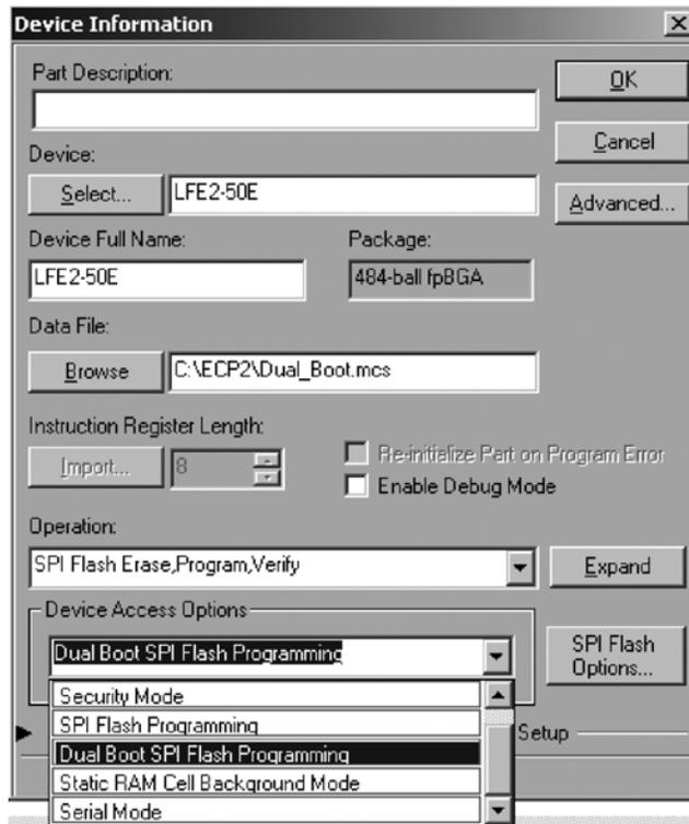
From the Device Options drop-down box select **Dual Boot SPI Flash Programming**. Then click on the **SPI Flash Options** button to open the SPI Serial Flash Device window (see Figure 15-5). In this window click on **Select** and choose the SPI Flash that’s mounted on the board.
