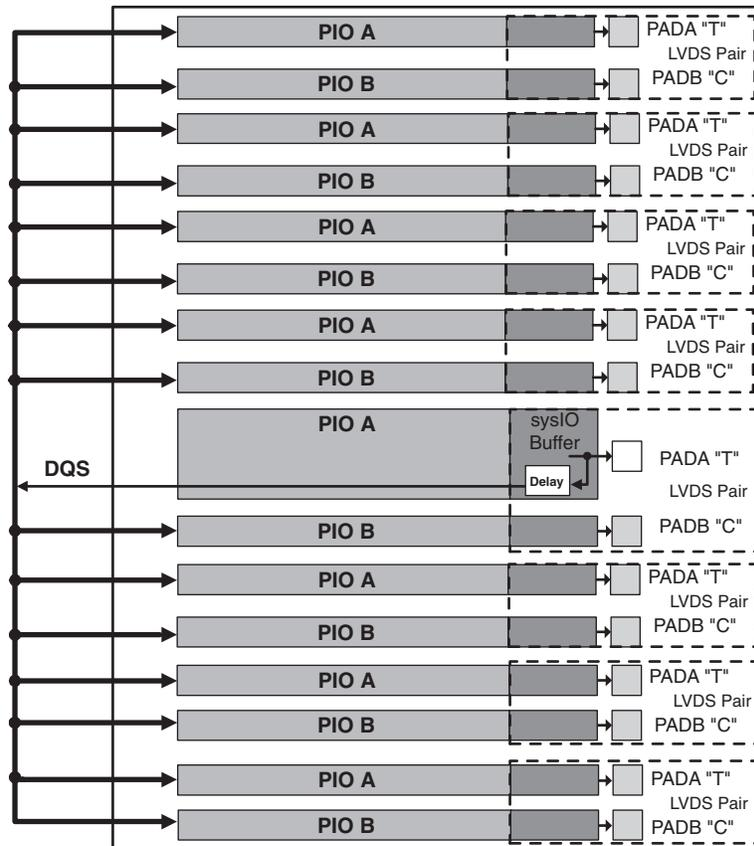
Figure 2-34. DQS Input Routing for the Bottom Edge of the Device
