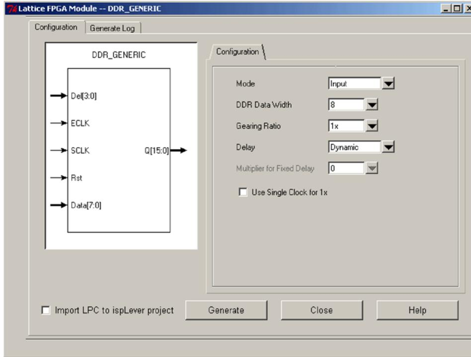
The user can change the Mode parameter to choose either Input, Output, Bidirection or Tristate DDR module. The other configuration parameters will change according to the mode selected. The Delay parameter is only available for Input and Bidirectional modes. Similarly the Multiplier for Fixed Delay parameter is only available when the Delay parameter is configured to Fixed.
